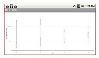
Figure 3. A whisker plot of temperature data showing min/max and 25th and 75th percentiles for each fridge.
