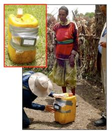
Figure 8: Researcher attaching the WuhaGize sensor, encased in a black box, to a water container. The inset shows the sensor attached to the water container.
