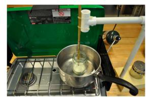
Figure 5: Flash heat pasteurization setup in the lab.
