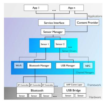
Figure 2: Generic architecture of the ODK Sensors Framework. *Service Interface* and *Content Provider* form the principal unified interface used by apps to communicate with the framework. *Sensor Manager* contains references to all available *Sensors. Channel Managers* are specific to communication channels and manage connections and data transfers with underlying hardware sensors.
