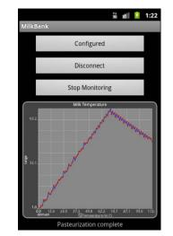
Figure 6: MilkBank application shows the temperature curve during the flash heat pasteurization process. This application is an example of real-time, time series use-case.
