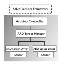
Figure 3: Architecture of the Arduino USB Bridge. The *Arduino Controller* facilitates communication between the Android framework and the *ARD Sensor Manager*, which talks to each sensor through its *ARD Sensor Driver*.
